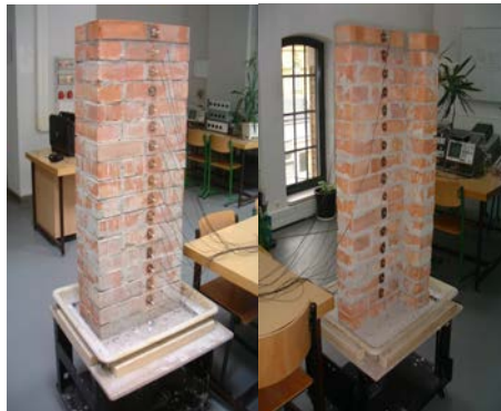
Fig. 3. Electrodes fixed to the both sides of the wall.
