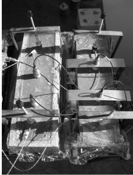
Fig. 3. Mounting acoustic emission sensors (on the left side sample from wood, on the right side sample from metal)
