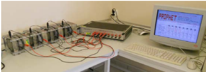
Fig. 9. PROOVE'it test set with connected four test chambers containing concrete samples 1/1, 1/2, 2/1,2/2 taken from road viaducts.
