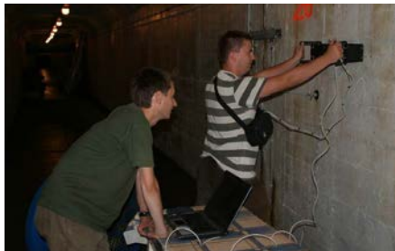
Fig. 4. Testing by means of ultrasonic tomograph.
