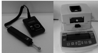
Fig.1. Measuring place (each measuring place consisted of five measuring points along wall height). Fig. 2. Moisture meter Uni with probe B50 (left) and drier-balance (right).
