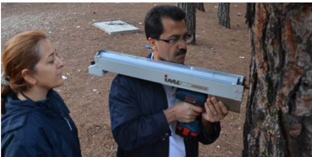
Figure 2. Resistograph (IML RESI F500-S) measurements at field
