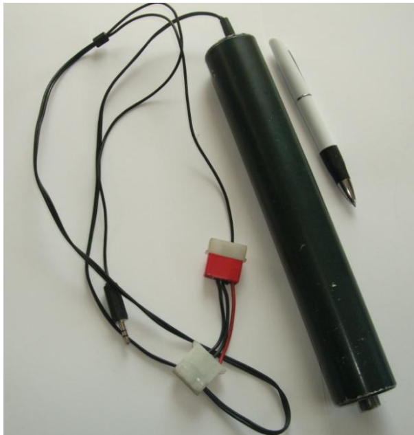
Photo1. The device for measuring of mechanical stresses
