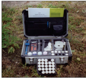
Fig. 2. Rapid Chloride Test kit for measuring chloride ion concentration in concrete.
