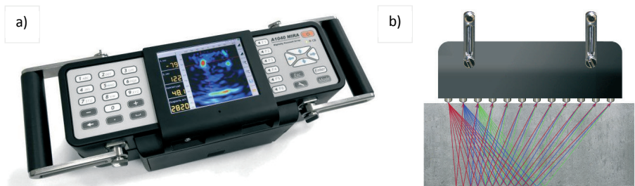
Fig. 3. Ultrasonic tomography: a) view of device b) the method of operation
