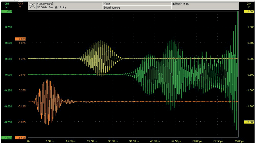
Figure 6. Example of one measured signal (both excitation and one scan) for time delay 16 \mu s
