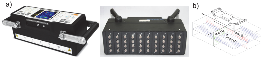
Fig. 1 Ultrasonic tomograph: a) view from the top and from the bottom, b) possible layout of displays
